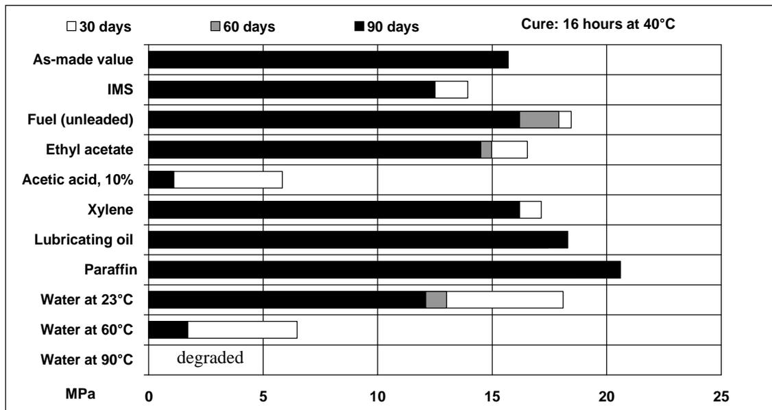
**Lap shear strength versus tropical weathering**
