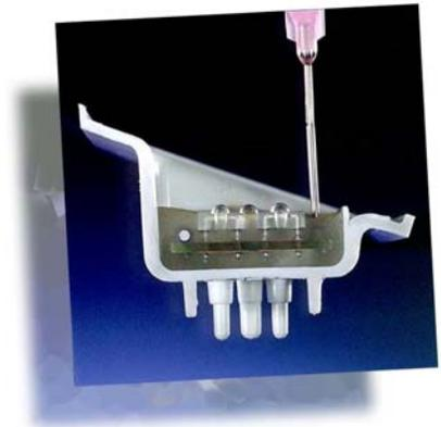
UV/visible potting to 15 mm with acrylate LCMs
