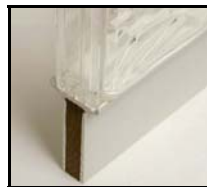
Glass block bonded to plastic with 4-20586
