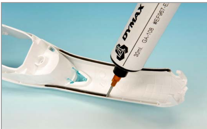
Dispensing gasket bead onto appliance handle
