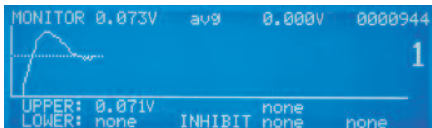
Monitor Screen – Shows 1st Pulse weld voltage exceeded limit.
