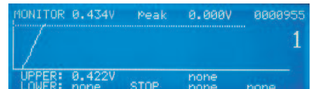
Monitor Screen – Shows weld voltage exceeding limit.
