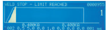
Run Screen – Shows termination of weld current during weld pulse.
