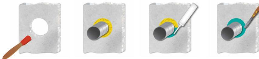
**Figure 5:** Typical tooling of penetration seals for DOWSIL™ FIRESTOP 700 Sealant.
