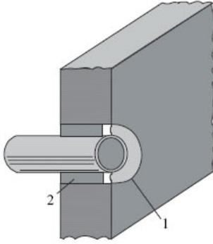
**Figure 3:** Illustration of centered penetration in a wall.
