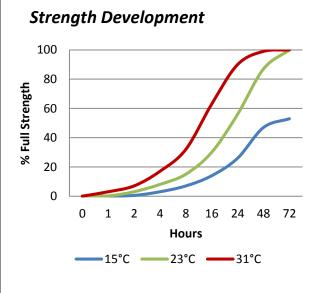
Graph shows typical strength development of bonded components. Lower temperatures will result in a slower cure time.
