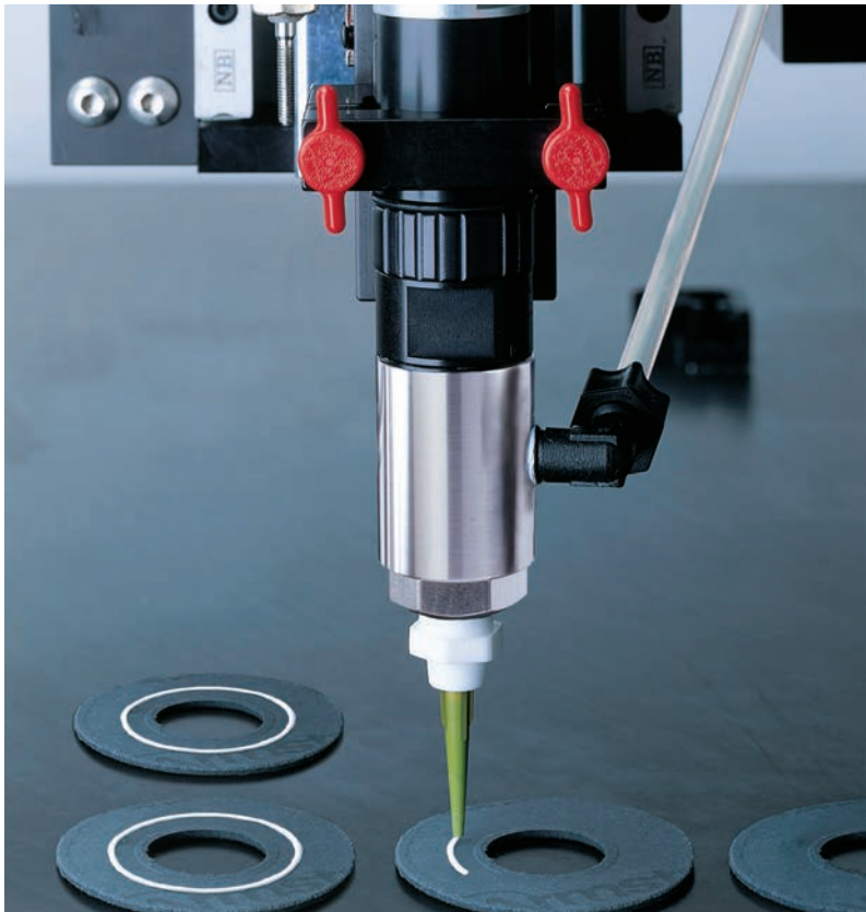
725D dispensing even bead of water-based adhesive.
