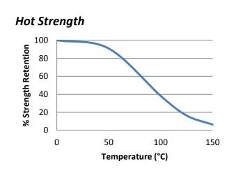
"Hot strength" shear strength tests performed on mild steel. Fully cured specimens conditioned to pull temperature for 30 minutes before testing at temperature. TA4205 can withstand higher temperatures for brief periods (such as for paint baking and wave soldering processes) providing the joint is not unduly stressed. The minimum temperature the cured adhesive can be exposed to is -40°C (-40°F) depending on the materials being bonded.
