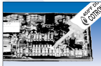
Duralco™ 125 Replaces Soldering on a Circuit Board
