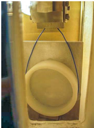
Figure 7. The panel and filled Teflon ring apparatus inside the environmental chamber prior to being tested.
