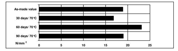
Tensile properties (ISO 527). (typical average values)- Cure 16hrs at 40 °C, tested at 23 °C
