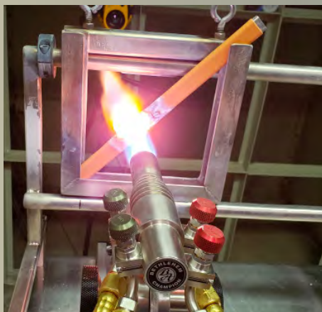
High-temperature torch exposure performed on HCR coated busbar test part
